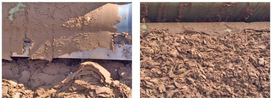
Sludge cake after treatment with Drewfloc™ 2481 polymer.
